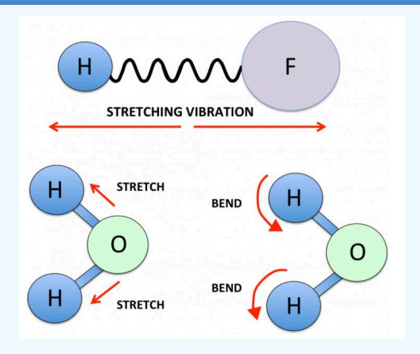
**Stretching and Bending occurs at distinct frequencies** Molecule must have a net dipole moment to exhibit IR spectra
